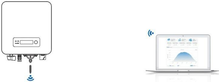
The operation information (generated energy, alert, operation status) of the inverter can be transferred to PC or uploaded to the server via Wi-Fi. You can register on the website.
