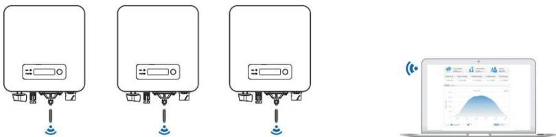
The operation information (generated energy, alert, operation status) of the inverter can be transferred to PC or uploaded to the server via Wi-Fi. You can register on the website.
